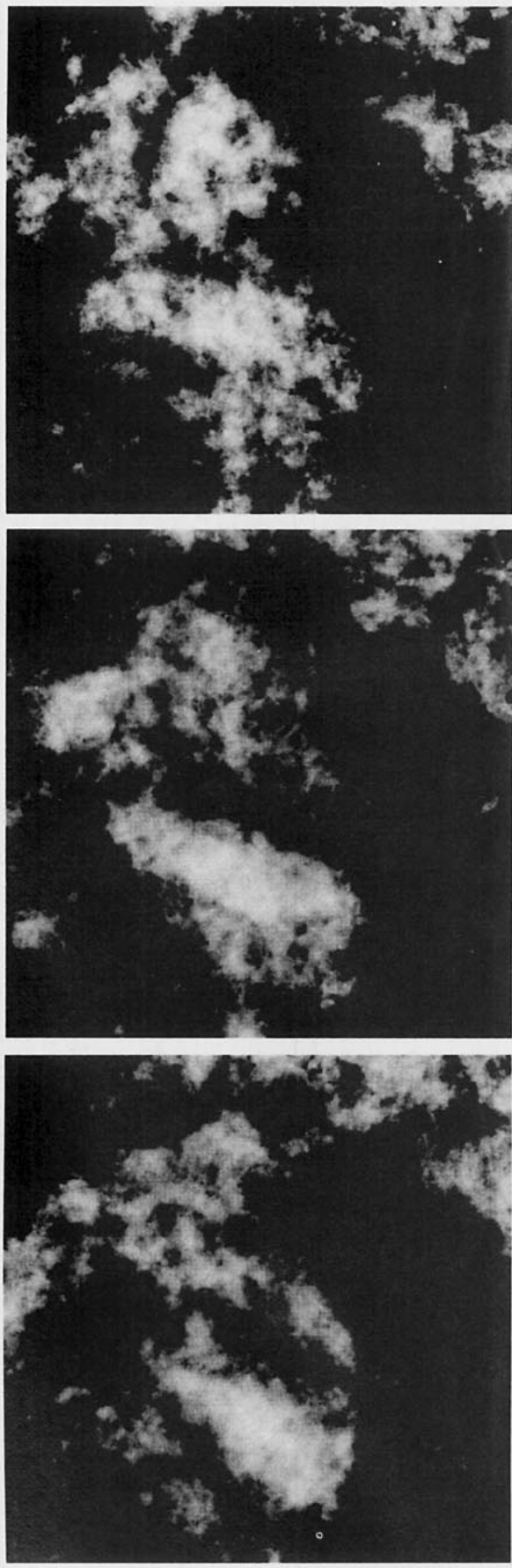
FIG. 10. (left) Model of the temporal evolution of an isotropic rain field on an 800 \times 800 point grid. The images are separated by a time equivalent to 80 pixels. The log rain intensity is shown by the shades in the figure—a black background (=no rain), with white being the most intense.
