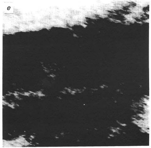
Fig. 3d, e Non self-similar (anisotropic scaling) FSP rain models on a 400 \times 400 point grid, using linear Generalized Scale Invariance with generators with off-diagonal elements to yield differential rotation. This results in differences in orientation of structures as functions of scale which is clearly perceived as cloud 'texture'. From Lovejoy & Schertzer (1985a).
